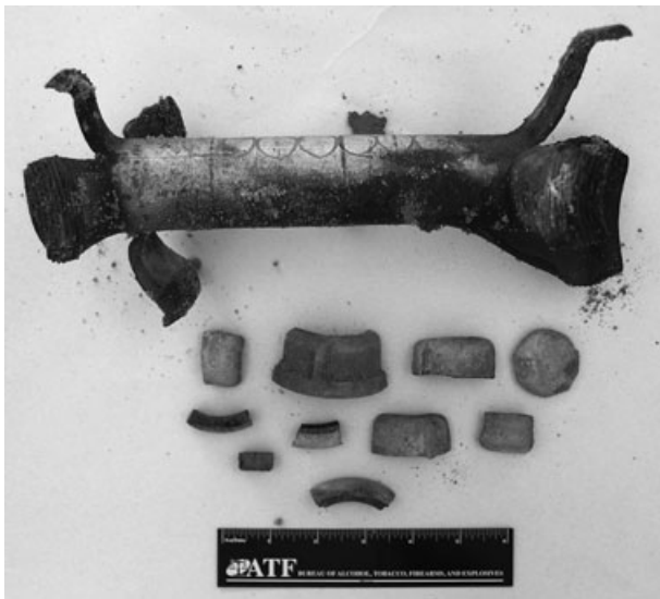
FIG. 9—The remains of a galvanized steel pipe bomb filled with Pyrodex and initiated with a pyrotechnic fuse. The fragments of this device were fumed in the field with cyanoacrylate and are shown after removal of multiple layers of Power First brand electrical tape that were applied to the exterior of the pipe nipple. Tape from a roll of Tartan 1710 was used to secure the secondary packaging for the explosive filler inside the pipe nipple.
